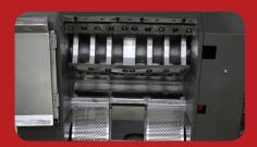
Wide open access to the front chamber for knife and screen cleaning
